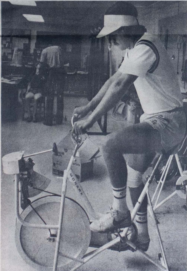
FITNESS PERFORMANCE —Terry Taylor, a 1972 graduate, gets firsthand experience at the Human Performance Laboratory at Northeast Missouri State University. Dr. Jerry Mayhew, lab director, sees how fast Taylor's pulse returns to normal after riding the stationary bicycle or ergometer with a tension belt that determines work load.
