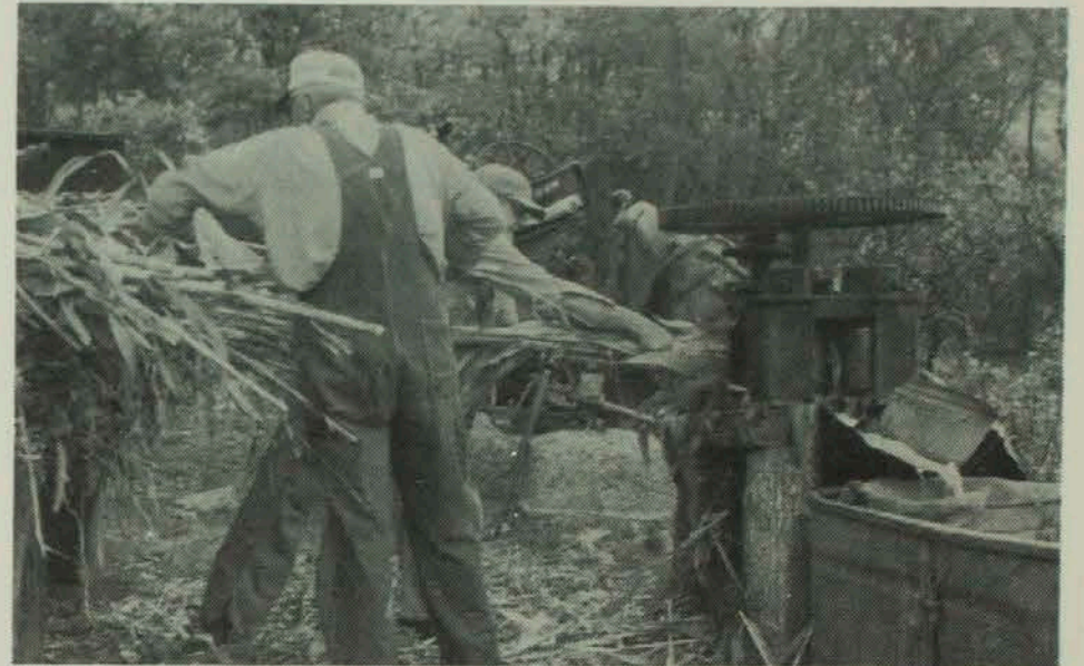
Marvin Mears and Butch Johnson run the cane stalks through the side of the press to squeeze out the juice. The power take-off on the tractor is used to run the cane press.
