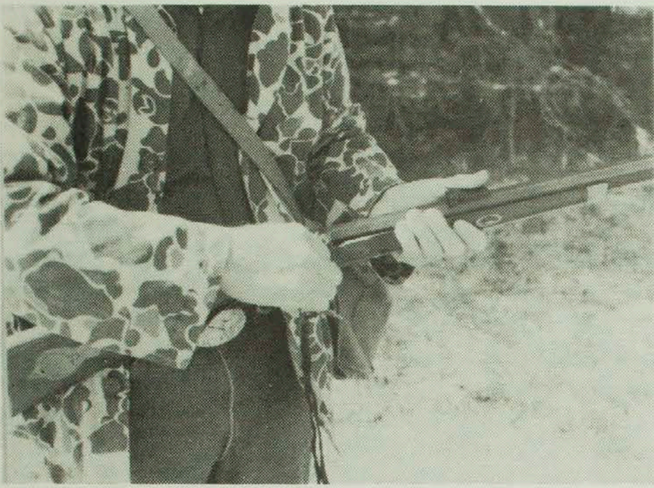
The first step of loading a muzzle-loader is firing a priming cap to burn the moisture out of the barrel.
