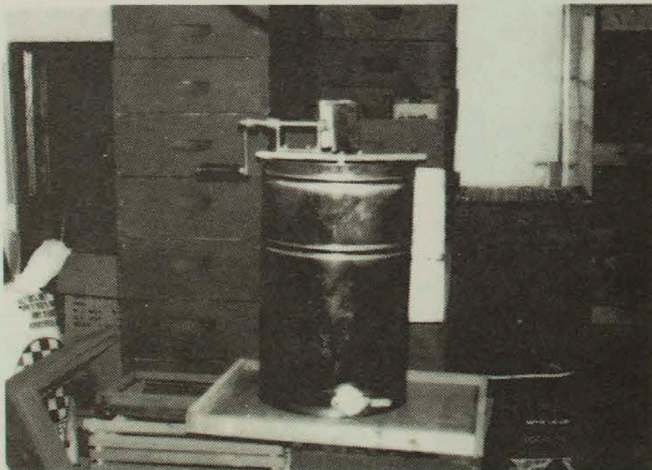
A handcranked honey extractor like the one pictured here is used to remove honey from its comb.
