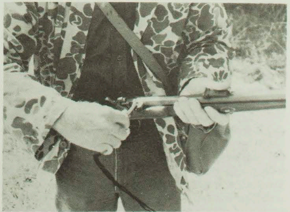
The last step before firing is placing a cap over the nipple and cocking the hammer back one click.
